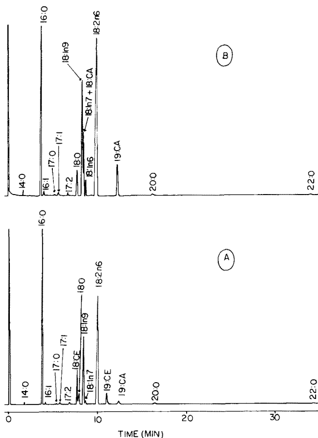
FIG. 1. GLC analysis of kapok seed oil fatty acid methyl esters on a Supelcowax-10 fused silica capillary column at 172 C. A, before hydrazine reduction, and B, after hydrazine reduction.
